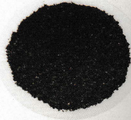
Type II – Coconut shell charcoal - granulated
